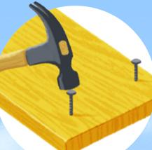
1. Hammer two nails into the end of a flat board, as shown. Place the nails at least 6 inches (15 cm) wider than the widest part of your paper airplane.
