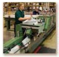
Printed signatures pass tbrougb a machine that collates them, adds the cover, and then "saddle stitches" (staples) them together. Each magazine is then trimmed of excess paper.
